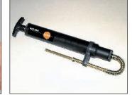
Smoke tester with oil, soot sheet for measuring soot in flue gas
