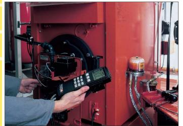
Heating technicians expect a lot from modern day flue gas analysers like the testo 300 M. Reliable results which can hold up to checks and comparisons have top priority. This is particularly important in the trades business since a burner is checked to see if it fulfills legal requirements. Advantage: All the measuring equipment incl. smoke tester in one case
