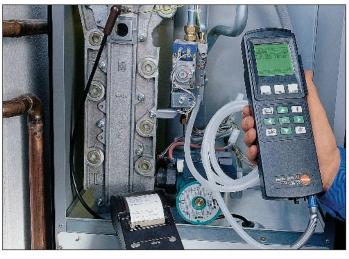
The affordable testo 300 M flue gas analyser is also a high standard pressure meter. It can measure absolute and differential pressures quickly and efficiently when used together with the practical hose connection set.
