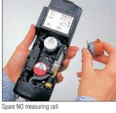
Quick and easy replacement of measuring cell by 0390 0074
