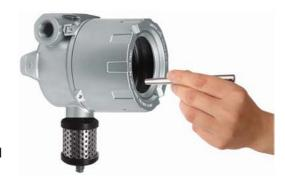
Magnetically operated switches allow the unit to be calibrated through the display window using the magnetic pen without the need to remove the cover from the unit.
