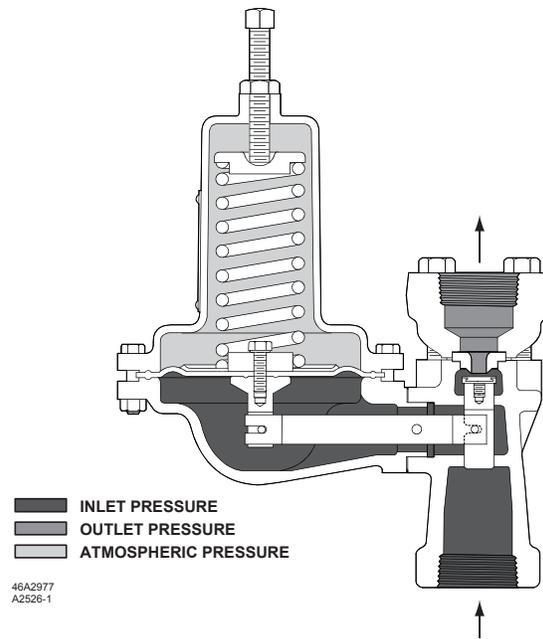
Figure 3. Type 630R Relief Valve Operational Schematic
