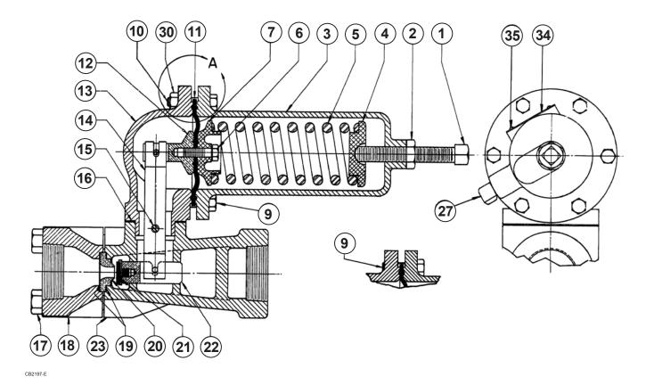
Figure 5. Spring Loaded Type 630 Regulator - High Pressure Construction
