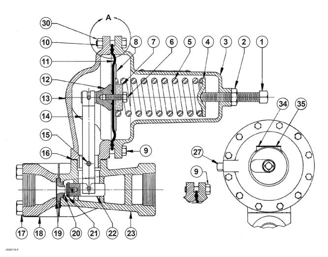
Figure 4. Spring-Loaded Type 630 Regulator - Low Pressure Construction
