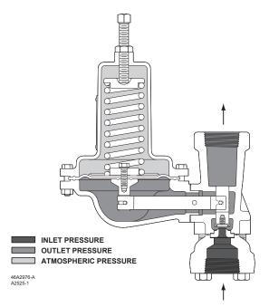
Figure 2. Type 630 Regulator Operational Schematic
