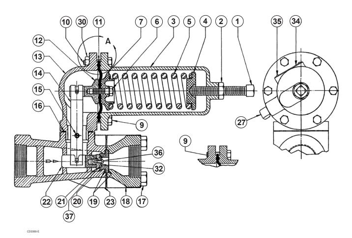
Figure 6. Spring-Loaded Type 630R Relief Valve High-Pressure Construction
